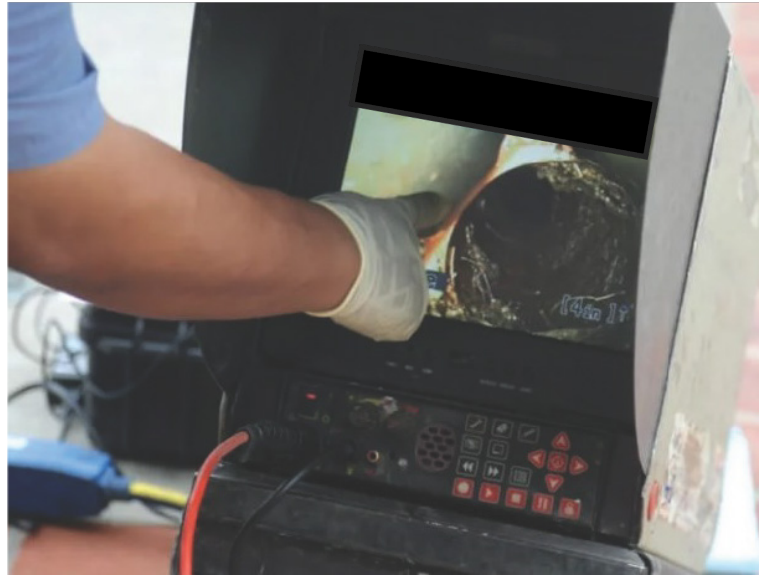
Pictured Above: a highly-trained technician uses high resolution CCTV equipment to inspect the inside of a sewer lateral.
